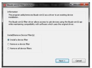
Select Install device filter. Make sure that the C232HM is the only FTDI device plugged in.
