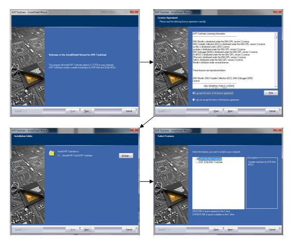
• In the last dialogue box select only the 8-bit tool chain for the Atmel AVR chip.
