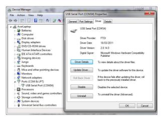
AVRDUDE requires the installation of the open source libusb driver in order to work with the FTDI chip. AVRDUDE uses the high speed SPI mode of the FTDI-232H chip in order to rapidly write and verify the flash memory on the AVR chip, it is no a so called bit-banger. To install the libusb driver go from:
